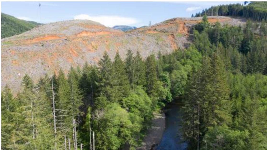
Exhibit 4. Effects of land clearing on erosion and shallow land sliding (Photo by Shane Anderson, circa 2018 from Chehalis River watershed approximately 1-mile upstream of FRE).
